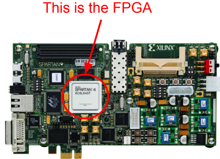
A Xilinx Development Board with a XC6LX45T FPGA (Spartan-6)
